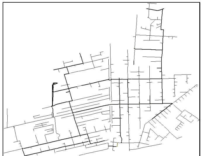
Fig. 4. Adopted urban medium voltage distribution network real topology, without the presence of elevated structures.
